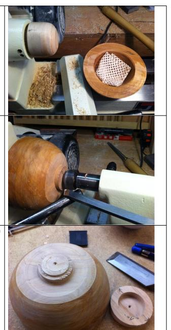
I chose to use epoxy for the gap filling properties and strength. Notice the small piece of masking tape covering the hole. This prevents the epoxy from leaking out. Apply the epoxy to the inside and mating surface of the donut and attach it to the bowl and apply some clamping pressure. Allow it to dry overnight and then the bowl is ready for a new tenon!
