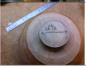
The depth of the hole should not penetrate the donut (I guess this makes is <u>not</u> a donut). My target depth is about 3/8" of an inch. Keep in mind that it needs to fit flat but not sloppy in order to get a solid glue joint. Chuck up the donut in the chuck and use a drill bit chuck in the tail stock with the proper size of Forstner bit. The final donut!
