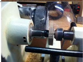
Determine the size of the hole to bore in the donut. In my case I chose a 1.50" hole so I could use a Forstner bit.
