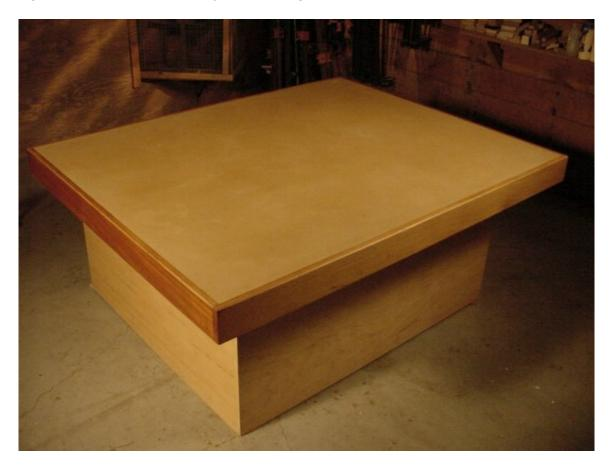
A torsion box is an excellent system to use for this type of table because it is very stable and has excellent resistance to warping, sagging, or bending. In addition, it weighs and costs less than using solid lumber.
