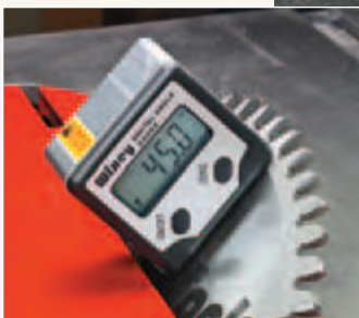
▲ Accurate Setup. A digital angle gauge helps guarantee an accurate miter.
