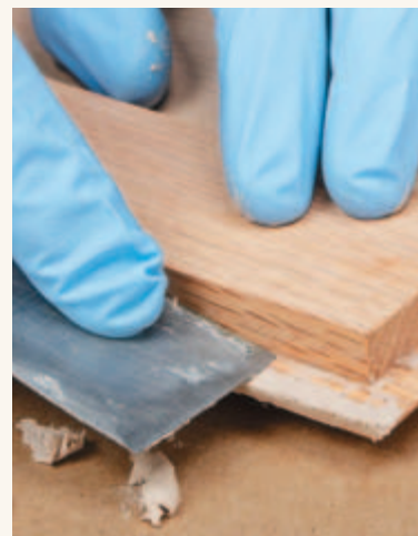
▲ Apply. You have about five minutes to apply the filler. Once it's hard, sand or rout it to shape.
