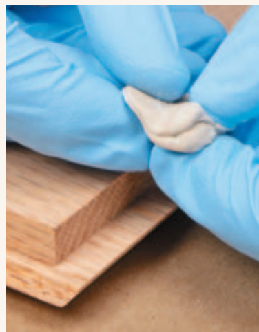
▲ Knead Together. Use your fingers to combine the two parts until the color is uniform.
