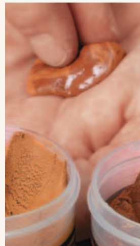
▲ Mix & Match. Mix colors of putty to create a custom match to your finished project.
