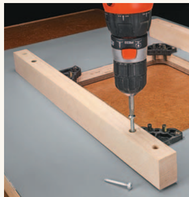
▲ Bracing for Support. Attach bracing to a sagging tabletop to keep it flat and rigid.
