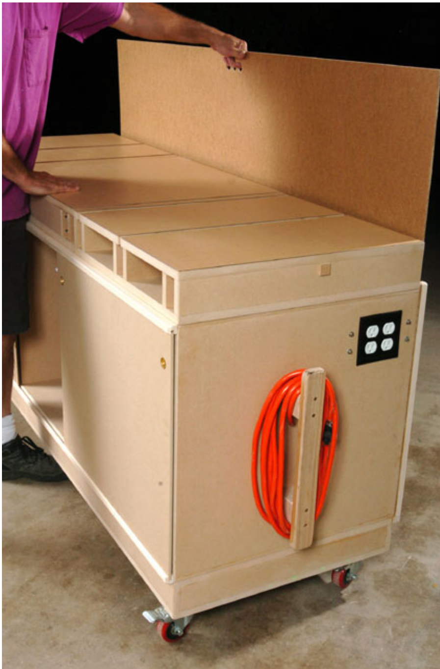
A sacrificial hardboard table-cover/drip shield stores in the back via slotted tracks. Glue-ups or careless banging on the top can be done without sullyng the finish.
