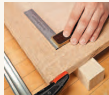
◀ Check for Square. Lightly tighten the clamps and make sure the assembly is square.
