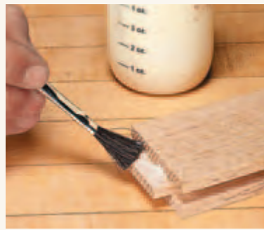
▲ Stub Tenons. With a brush, apply a thin coat of glue to just the cheeks of the stub tenons.
