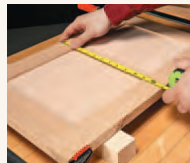
◀ Across the Middle. Compare the middle to the ends to see if the stiles are bowed.
