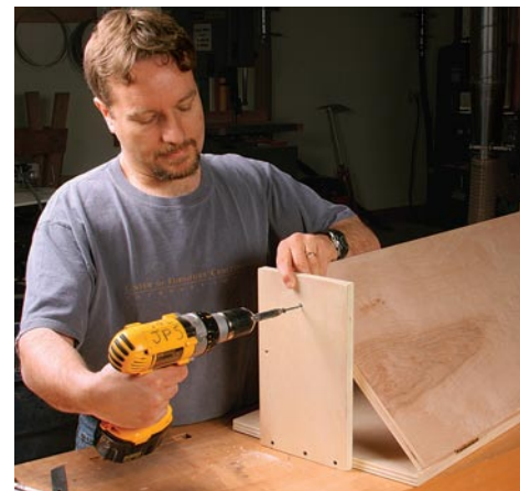
Set up the angle. Once the leaves are hinged and the uprights are screwed to the lower leaf, use a bevel gauge to set the angle (left), and screw through each upright to lock the upper leaves (right).
