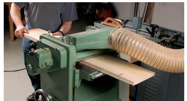
Plane it smooth. Next, with the steps facing down on the bed, he runs the board through the planer until the board has been planed across its length. Then he flips the board over and gradually removes the steps.
