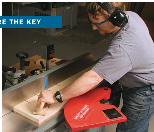
Plane it smooth. Next, with the steps facing down on the bed, he runs the board through the planer until the board has been planed across its length. Then he flips the board over and gradually removes the steps.
