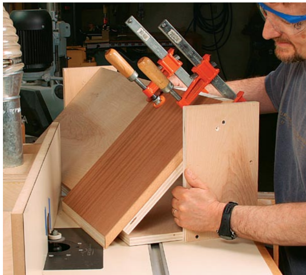
Set up the angle. Once the leaves are hinged and the uprights are screwed to the lower leaf, use a bevel gauge to set the angle (left), and screw through each upright to lock the upper leaves (right).
