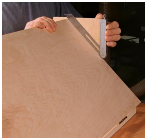
Set up the angle. Once the leaves are hinged and the uprights are screwed to the lower leaf, use a bevel gauge to set the angle (left), and screw through each upright to lock the upper leaves (right).
