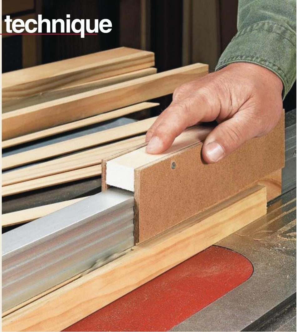
▼ Use a combination blade (left) or rip blade to cut thin strips.
