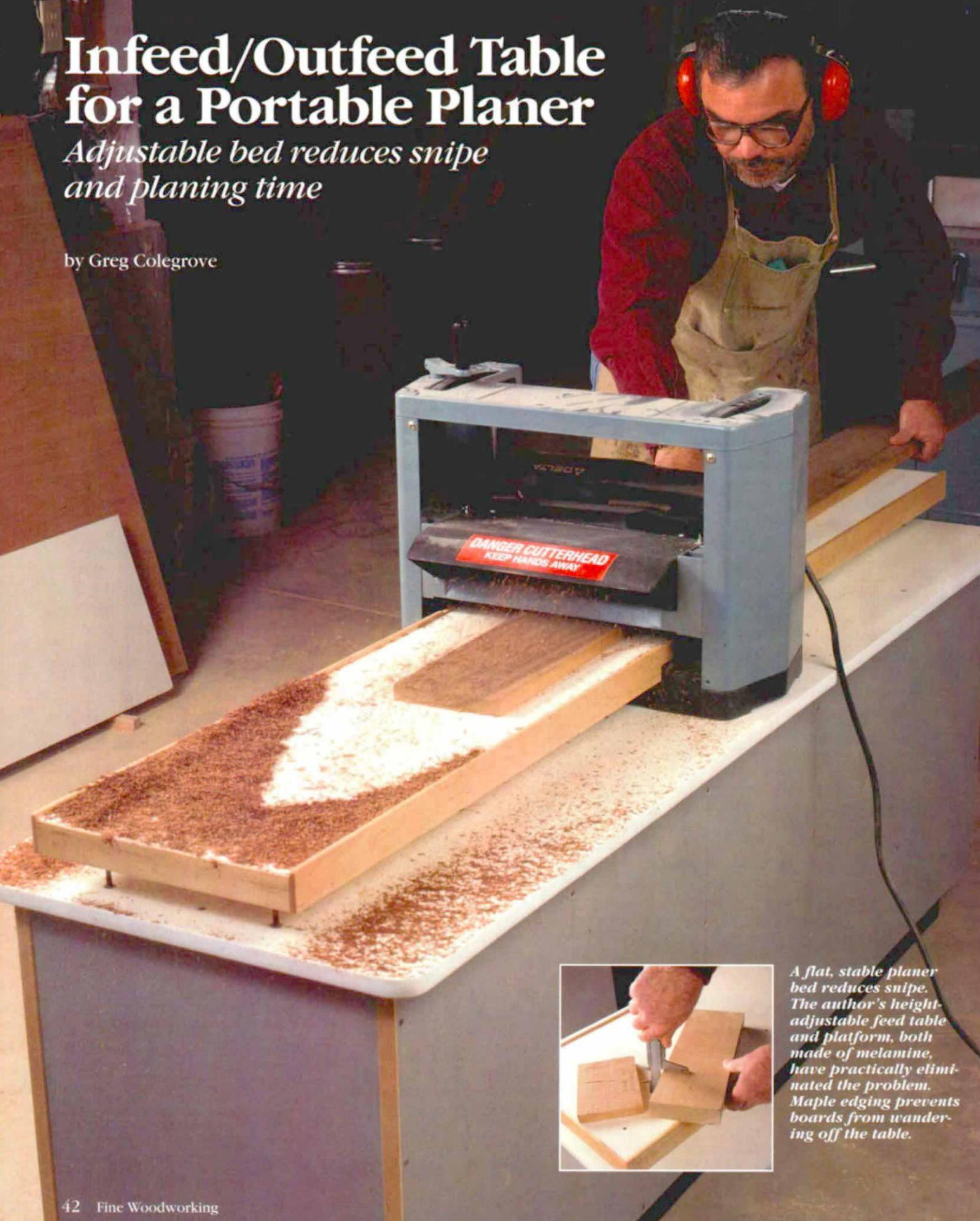
*A flat, stable planer bed reduces snipe. The author's height-adjustable feed table and platform, both made of melamine, have practically eliminated the problem. Maple edging prevents boards from wandering off the table.*
