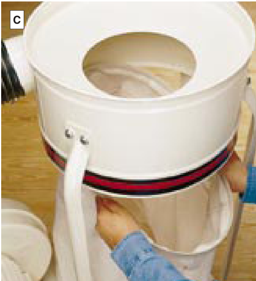
Rather than a traditional bag clamp, the Jet DC-1100 has a spring-steel hoop stitched into the bag's mouth for effortless bag removal and installation.
