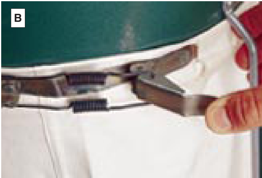
The release lever on the Grizzly G8027's bag clamp bent easily when closing it. Since our test, a Grizzly spokesman told us they would improve the clamps.
