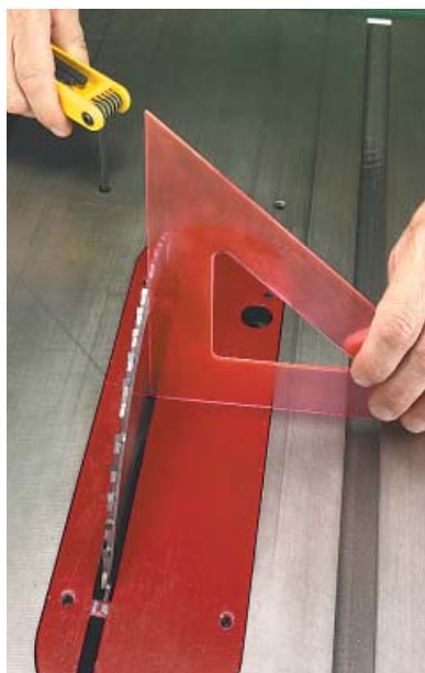
◀ Setting Stops. A drafting triangle can be used for checking the 90° (left) and 45° (right photo) settings.
