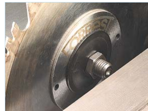
▲ Stiffener. Although it reduces the depth of cut, a blade stiffener is an inexpensive way to reduce saw blade vibration.
