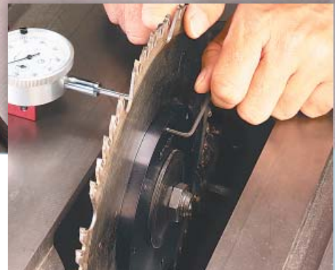
▲ Zero Out the Runout. With this saw blade truing disc, you can reduce the runout of your table saw to a minimum.
