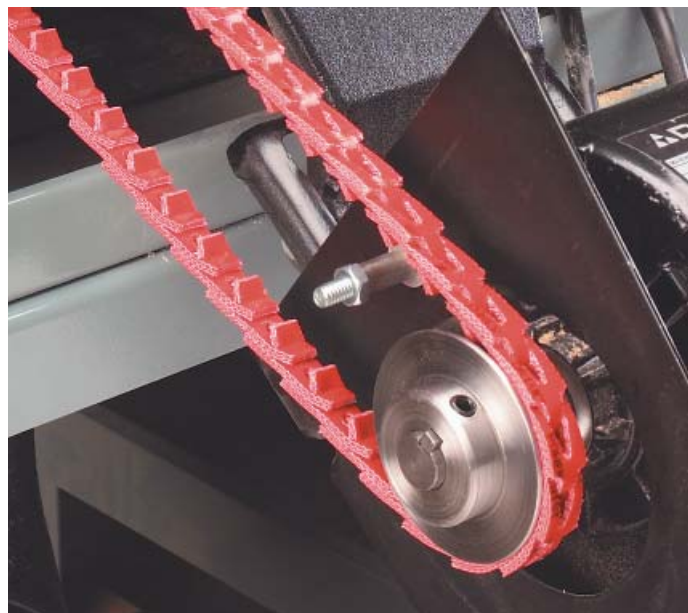
◀ Belts & Pulleys. A link belt and machined pulleys will make your saw run smoother.
