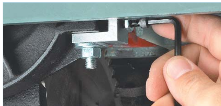
▲ Trunnion Alignment. For easy and precise trunnion alignment, nothing beats the Precision Alignment and Locking System (PALS).
