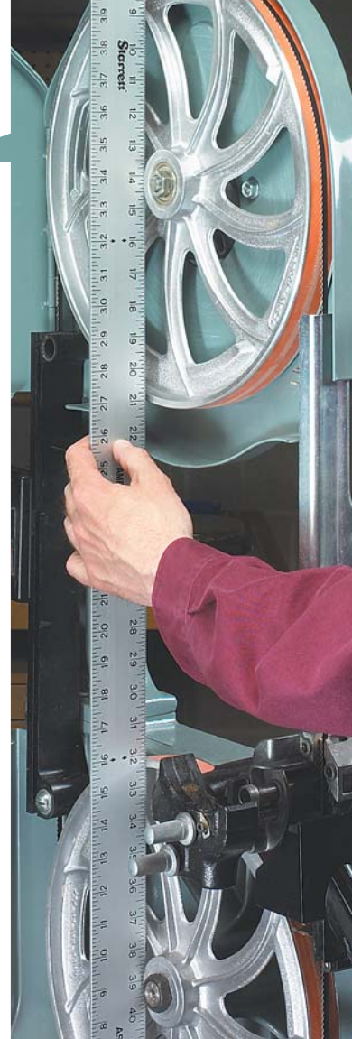
▲ Wheel Alignment. Adjust the wheels either by tilting the top wheel (detail 'a') or by repositioning one of the wheels (detail 'b').
