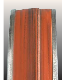
▲ Tire Wear. The ridge on this tire was caused by setting the blade tension too high.
