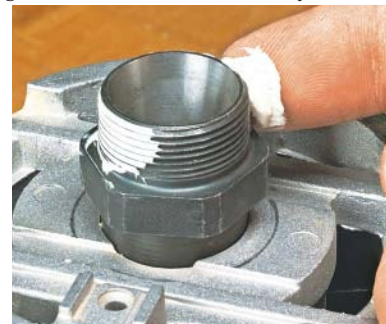
▲ Lubrication. A coat of white grease on the arbor threads ensures hassle-free bit changes.
