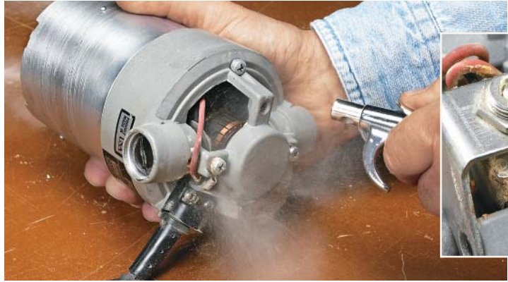
▲ Blow Out the Dust. It's unavoidable — the inside of a router traps dust. But all it takes to clean out the motor and the important electrical connections is a blast of compressed air.
