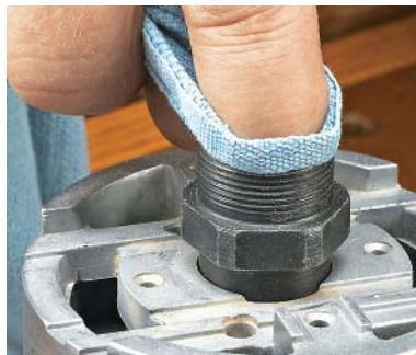
▲ A Snug Fit. The accumulated dust and debris in the arbor socket should be wiped or blown out.
