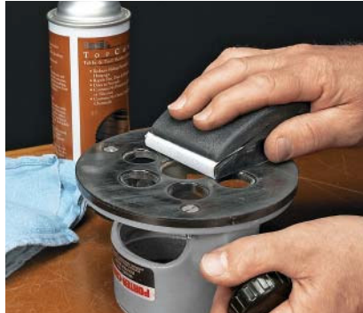
▲ Keep It Smooth. Lightly sanding the base plate with fine-grit sandpaper will keep it smooth and level.
