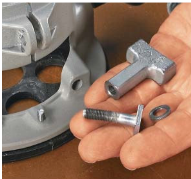
▲ Out With the Old. The bolt is bent, the knob chewed up and the threads are wearing out.
