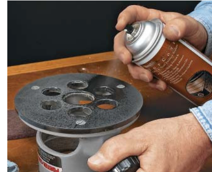
▲ Make It Slick. A light coat of surface lubricant will make the base plate slide effortlessly.
