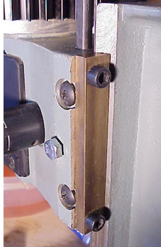
Adjusting the slides is one of the critical parts of setting this machine up for accurate operation.
