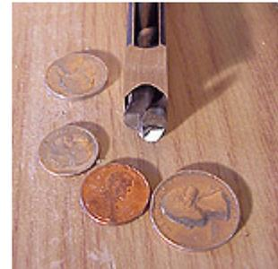
(Top) The bit-to-chisel clearance is crucial to proper operation and life of the parts.
