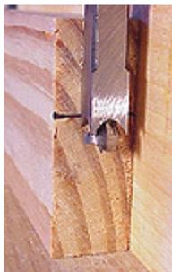
When setting depth, we have to remember the bit protruding ahead of the chisel.
