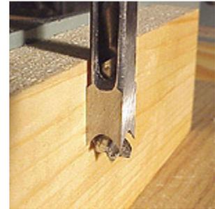
Using the fence itself to square the chisel is fast and very accurate.
