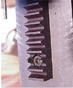
Don't forget to clean the teeth of the gears that move the head up and down.
