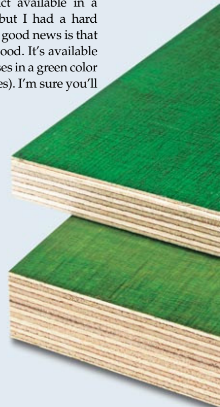
▲ Water-Resistant. A thin phenolic film protects the faces. You’ll want to seal the edges for exterior use.
