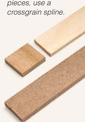
▲ Long Miters. A "capped" plywood (upper) or a hardboard (lower) spline work well for long miter joints.
